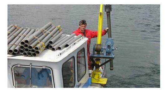
The advantage of this system is that it operates in any water depth. The maximum lenght of the core barrel is 3 m, and a PVC liner with a diameter of 70 mm is mounted inside.
