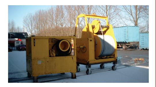
This winch is hydraulic driven with a separate hydraulic unit with a slip ring. The hoisting/electrical cable has a length of 1,000m (diameter 30 mm). The breaking strength is 50 tons.
