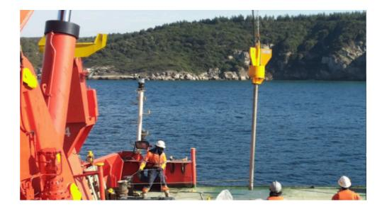
The advantage of this system is that it operates in any water depth. The maximum length is limited to the mounting length of the vessel. A PVC liner with a diameter of 98 mm is mounted inside to retrieve undisturbed samples.
